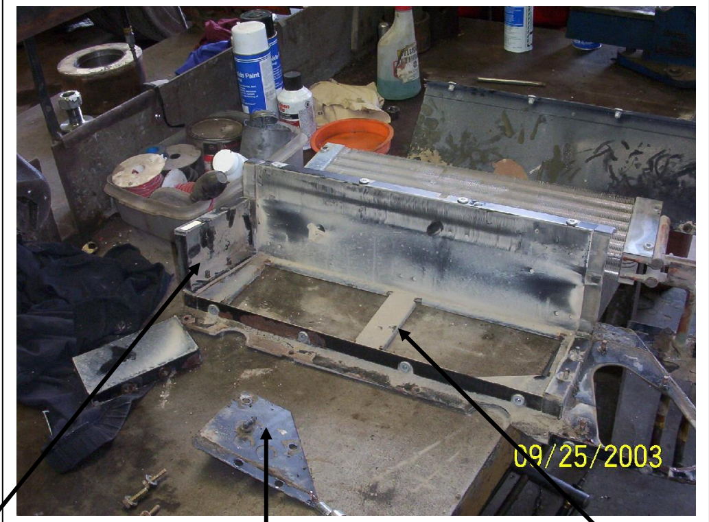
End cap flipped over so it cups out to accommodate the evaporator coil
